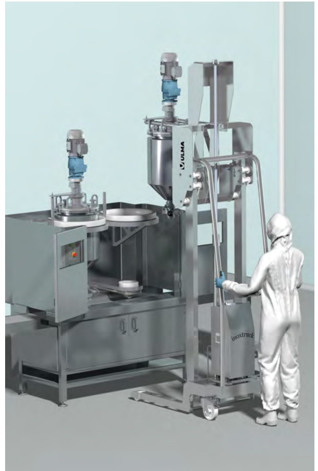
EMS lifter - reactor handling
