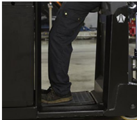
Suspended operator's platform.
