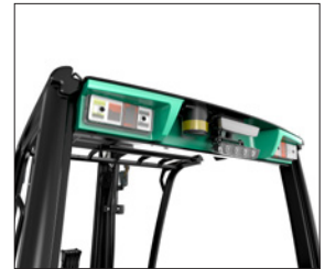
LED working lights, 2 front and 1 rear.
