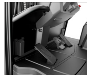
Dual pedal system - forward and reverse. (Option)
