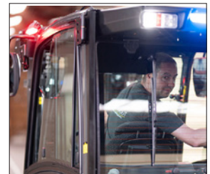
Blue point and red line safety lights
